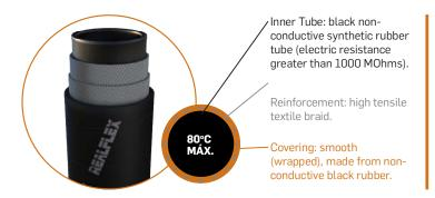
**APPLICATION**Hose used to protect electrical cables and to insulate and chill cables and spot welding machines
